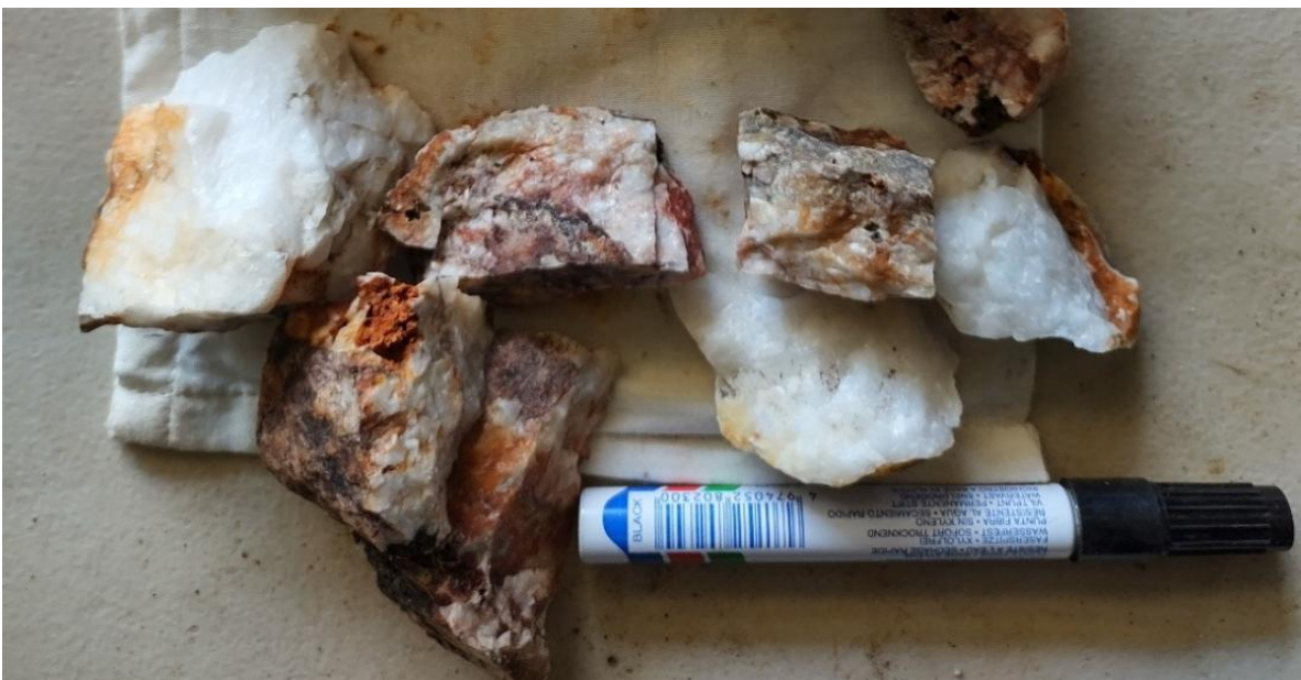
Figure 5: Sample 3017027, the best Ag sample (153ppm) has good Au W Bi in centimetre-scale sulfide-quartz veins in brecciated buck quartz that is otherwise barren.
