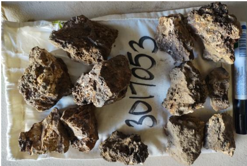
Figure 7: Sample 3017053, the best bismuth sample has 2660ppm Bi & 18.05% Fe, high grade Au, Ag and anomalous Cu & Pb in a breccia of rock and quartz with sulfide-filled cavities. This texture is the best visual guide to mineralisation.
