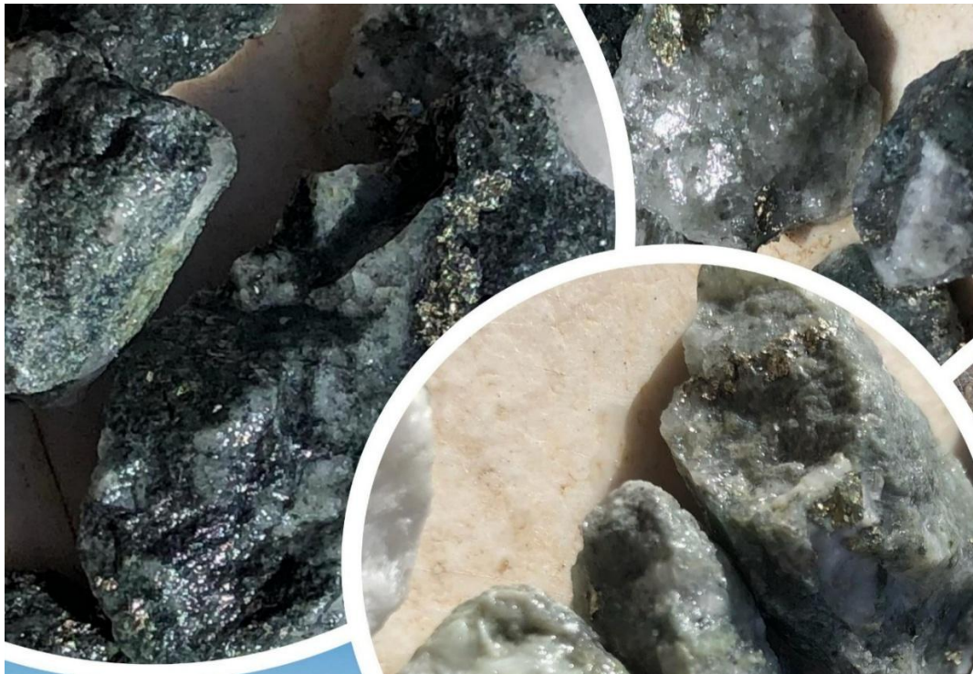
Figure 7: The Sulphides in drill chips, BGM, 2018 4
