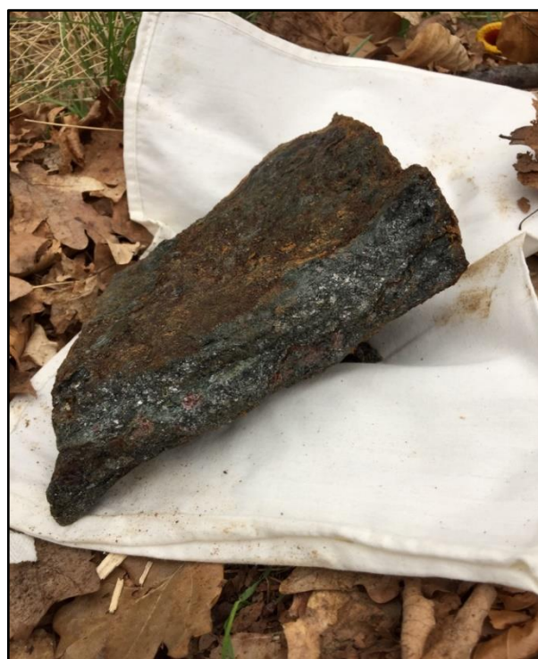
Grab sample of garnet mica schist from waste dump showing high grade cobalt mineralisation.
