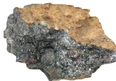
Figure 3: Grab sample of garnet mica schist from waste dump showing cobalt sulphide mineralisation.
